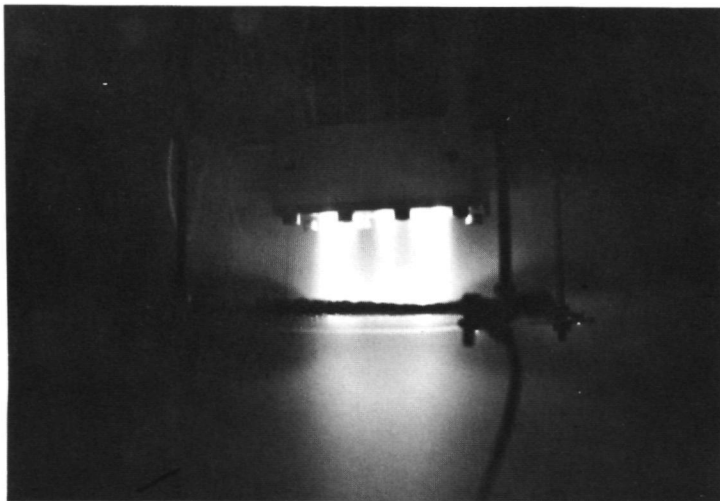
Figure 5.2: A photograph of the high voltage high pressure slit nozzle discharge, expanding a \text{N}_2/\text{H}_2 mixture. On top the five electrodes can be seen. The discharge starts at the nozzle and ends on the grid. The far infrared beam is guided in between.
