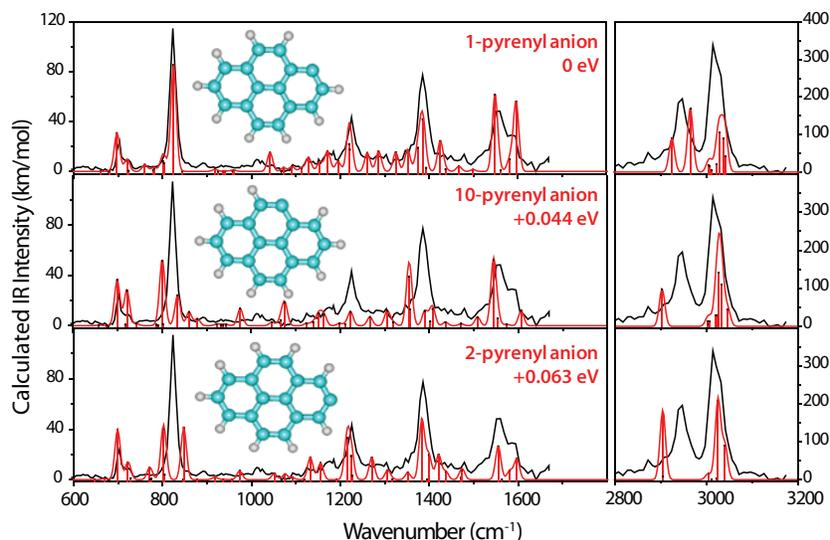
**Figure 5.** Gas-phase IRMPED spectrum of the pyrenyl anion (black) using 1-pyrene carboxylic acid as precursor compared to theoretical spectra (red) of the singlet 1-pyrenyl, 2-pyrenyl and 10-pyrenyl anions. The units of  $\text{km mol}^{-1}$  refer to the stick spectra only.
