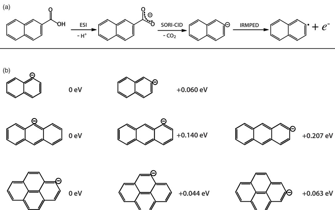
**Figure 1.** (a) Schematic showing the generation of the 2-naphthyl anion from its 2-naphthoic acid precursor. IR multiple-photon induced electron detachment (IRMPED) is used to detect light absorption as function of the IR wavelength applied (see text for details). (b) Isomeric structures of deprotonated naphthalene, anthracene, and pyrene. Relative energies with respect to the lowest-energy singlet isomer calculated at the B3LYP/6-31+G(*d, p*) level of theory are indicated.
