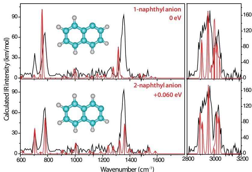
**Figure 3.** Gas-phase IRMPED spectrum of the naphthyl anion (black) using 2-naphthoic acid as precursor compared to theoretical spectra (red) of singlet 1-naphthyl anion and 2-naphthyl anion. The units of  $\text{km mol}^{-1}$  refer to the stick spectra only.
