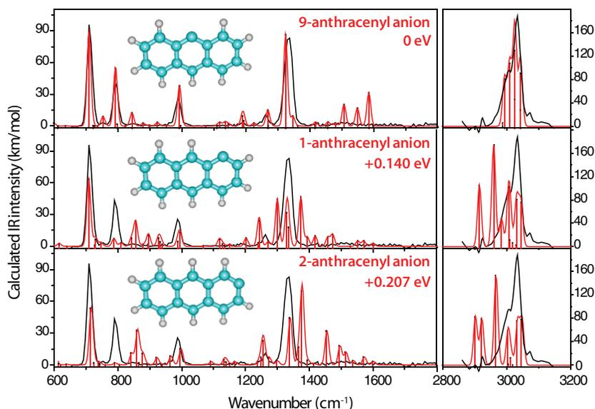
**Figure 4.** Gas-phase IRMPED spectrum of the anthracenyl anion (black) using 9-anthroic acid as precursor compared to theoretical spectra (red) of the singlet 1-anthracyl, 2-anthracyl and 9-anthracyl anions. The units of  $\text{km mol}^{-1}$  refer to the stick spectra only.
